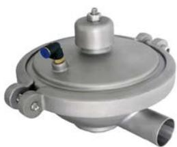
The Saniquip SCP constant pressure valves offer a simple method of maintaining a constant inlet or outlet pressure in process lines. They are remotely controlled using compressed air and require only a compressed air regulating valve and pressure gauge in the line for operation. An internal diaphragm and plug assembly reacts to any change in product pressure adjusting its position so that the preset pressure is maintained.
